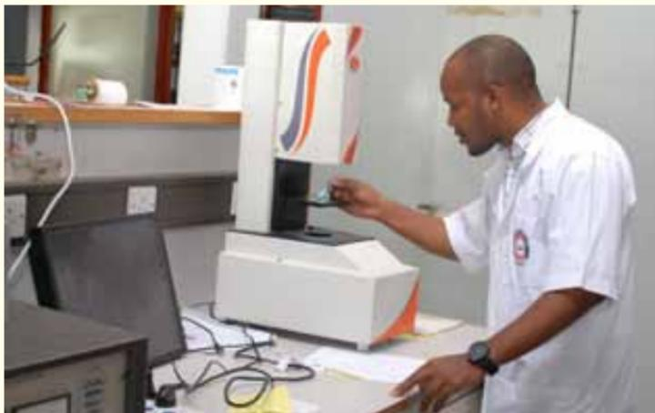
*Engineer testing insulation thickness of a cable in the Electrical Laboratory*
